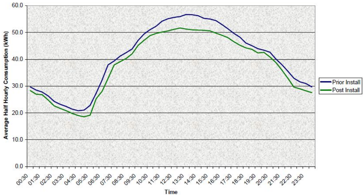
Figure 1: Average consumption by half hour comparing pre and post Powerstar install
